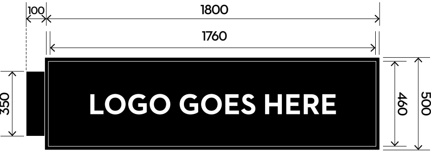
CL: CANTILEVERED LIGHT BOX ELEVATION: Face Dimensions SCALE: 1:20 @ A3 SIGN ID: CL.01, CL.02, CL.03, CL.04, CL.05, CL.06
