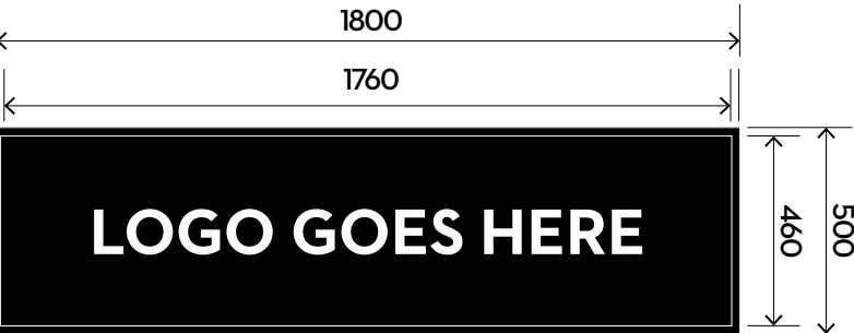
AE: ABOVE ENTRY RETAIL LIGHT BOX ELEVATION: Face Dimensions SCALE: 1:20 @ A3 SIGN ID: AE.01, AE.02, AE.04
