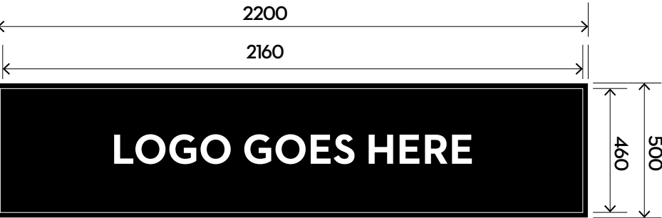
AE: ABOVE ENTRY RETAIL LIGHT BOX ELEVATION: Face Dimensions SCALE: 1:20 @ A3 SIGN ID: AE.03
